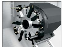
Both ST-10 models are equipped with a 12-station turret (BOT or VDI) that indexes in 0.5 seconds to reduce cycle times.
